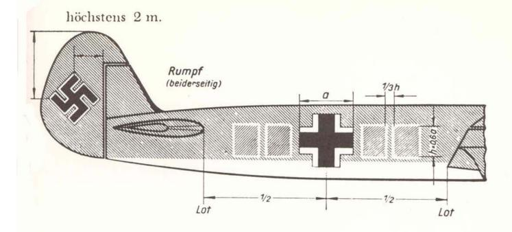
Location of military markings and codes on fuselage and empennage of front-line aircraft. Positioning of the *Hakenkreuz* on the rudder was purely diagrammatic, the main implication being that the distance from the mid-point of the marking to the tip of the fin/rudder was not to exceed two metres.
