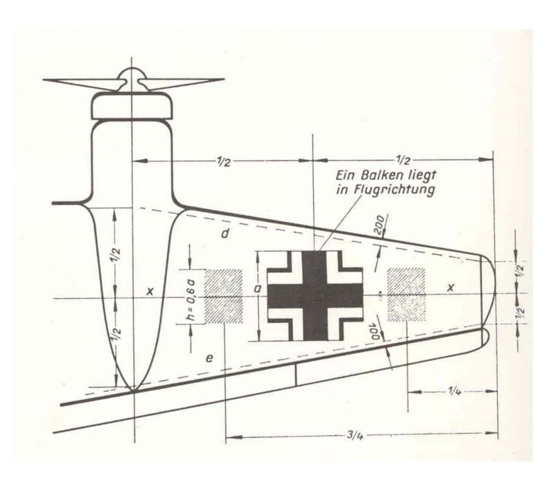
Balkenkreuz placement on wing lower surfaces for twin engine aircraft
